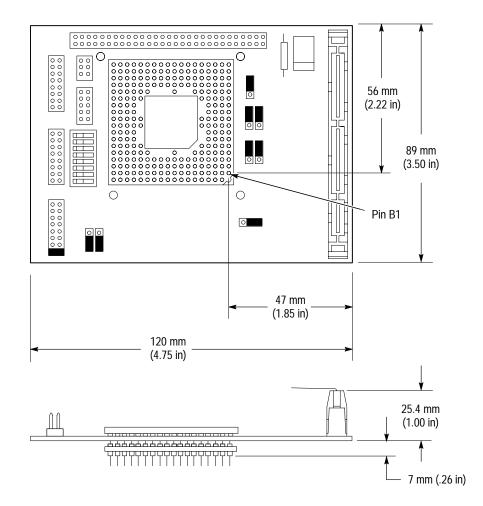
Figure 3-2: Dimensions of the low-profile probe adapter
