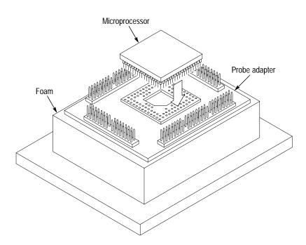
Figure 1–11: Placing a microprocessor into a PGA probe adapter
