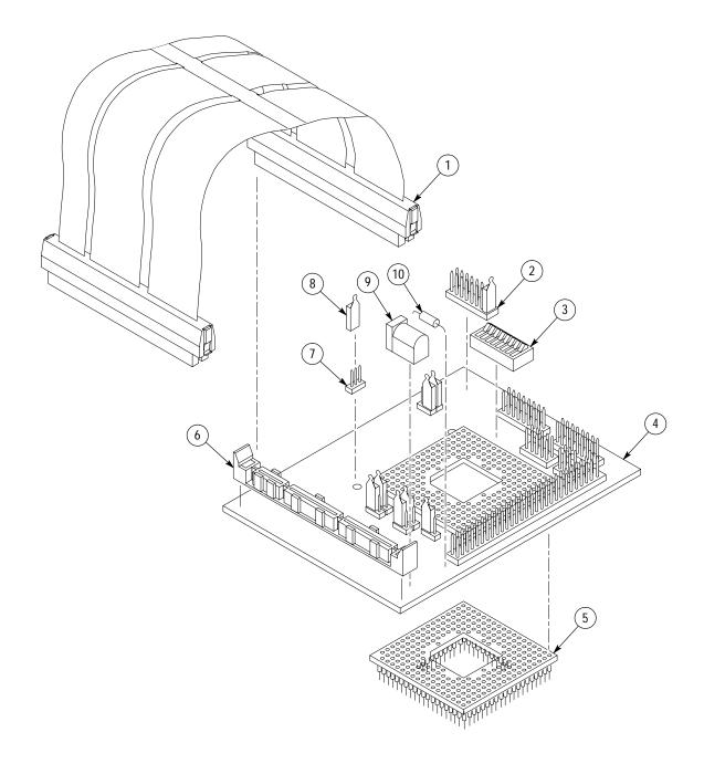
Figure 6–1: 68360 low-profile probe adapter exploded view
