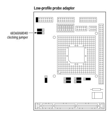
Figure 1–3: 68360/68040 clocking jumper location
