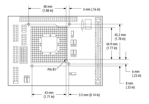
Figure 3-3: Tie-down hole placement on the low-profile probe adapter
