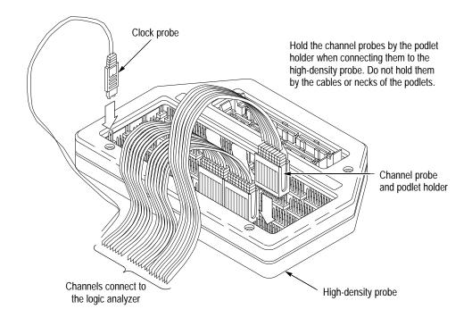
Figure 1–9: Connecting channel and clock probes to a high-density probe
