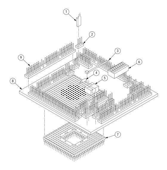
Figure 6-2: 68360 conventional probe adapter exploded view
