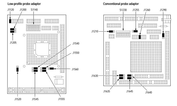
Figure 3–1 shows the locations of the jumpers and switches on the probe adapters. Refer to Table 3–1 for descriptions of each jumper.
