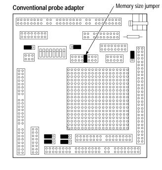
Figure 1–1: Memory Size jumper location
