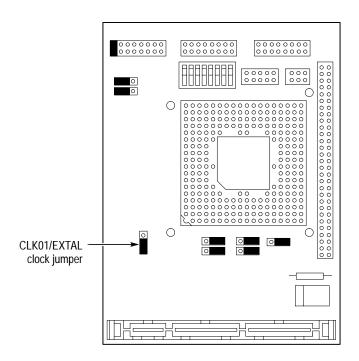
Figure 1–4: CLK01/EXTAL clock jumper location
