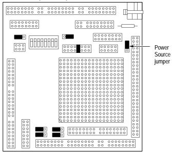
Figure 1–6: Power Source jumper location
