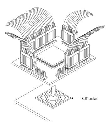
Figure 1–13: Placing a PGA probe adapter onto the SUT
