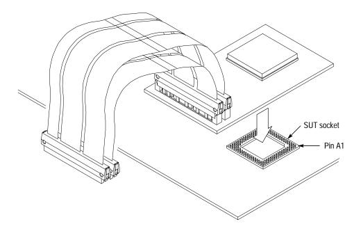
Figure 1-8: Placing a PGA probe adapter onto the SUT
