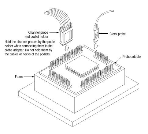
Figure 1–12: Connecting probes to a PGA probe adapter
