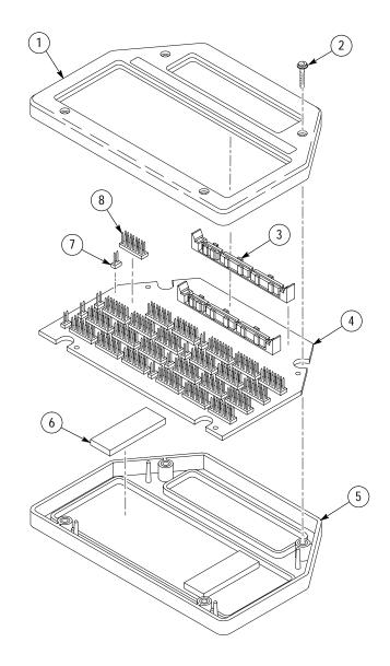
Figure 6–3: 192-Channel High-Density Probe exploded view
