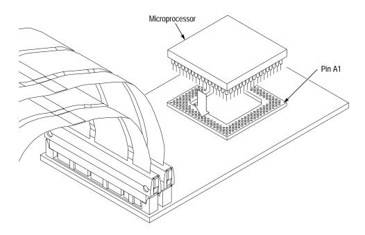
Figure 1–7: Placing a microprocessor into a PGA probe adapter
