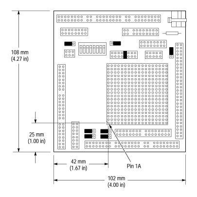
Figure 3-4: Dimensions of the conventional probe adapter
